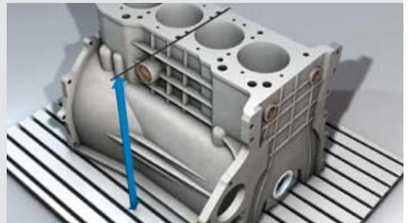
4. Observe the minimum dimensions of engine block and cylinder head according to the manufacturer's specifications, as well as the specified head gasket thickness.
