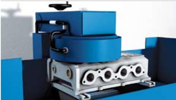
3. Remove any gouging, component distortions, grooves or scores, e.g. by surface grinding in a specialist workshop.
