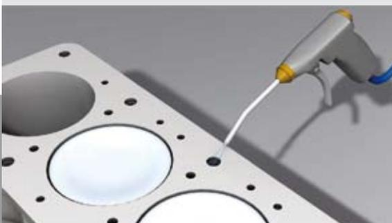
5. Clean the bolt hole threads, and remove any contamination, oil and water, e.g. with a blast of compressed air.
