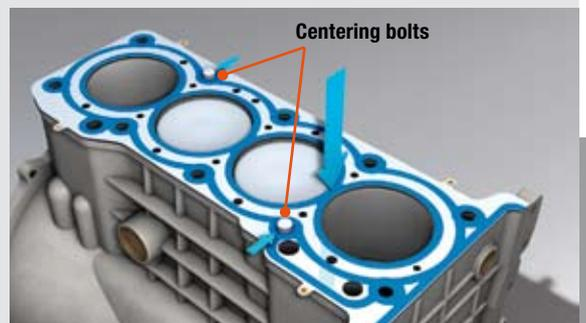
6. Position the head gasket accurately on the engine block. Do not use any additional sealing compounds, grease or oil.
