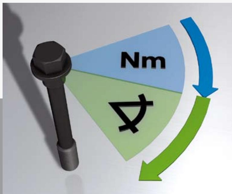
Torque-angle method using pretorque and tightening angle.
