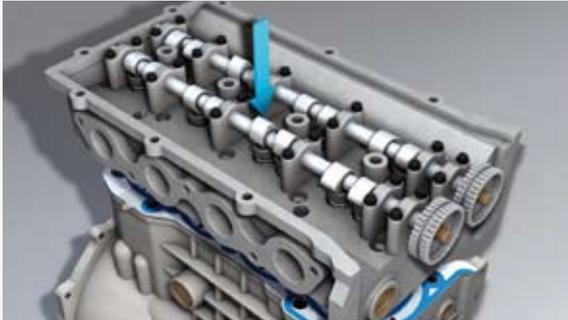
**7.** Fit the cylinder head, and take care not to damage the head gasket during assembly.
