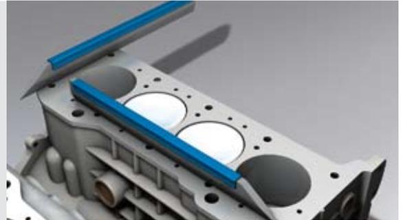
2. Use a straightedge to check the surface flatness; longitudinally and transversely.
