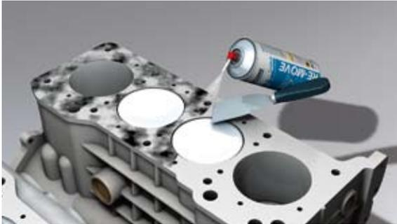
1. Carefully clean the sealing surfaces of engine block and cylinder head – dirt and gasket remnants on the surfaces are a frequent source of trouble.
