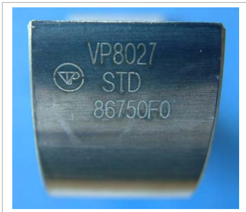
Laser marking on a new bearing (Main bearing for BMW Mini Cooper S 1.6L)
