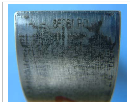
Used bearing shows how laser marking does not interfere with the back contact
